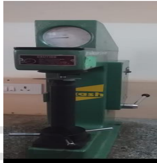
Fig 16: Rockwell hardness test machine
